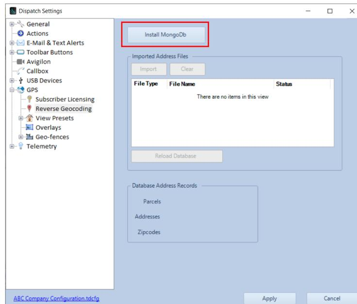
To install MongoDB, press the
