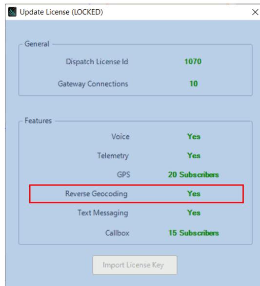
If a green **Yes** is to the right of Reverse Geocoding then the reverse geocoding license is installed properly.
