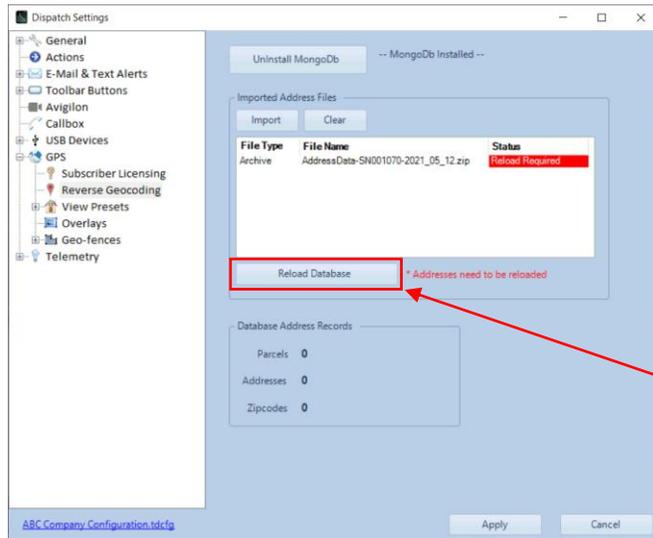
Press the **Reload Database** button to reload the Reverse Geocode Database.
